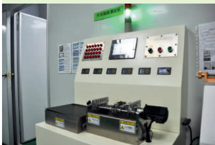
LIFE CYCLES TESTING MACHINE
