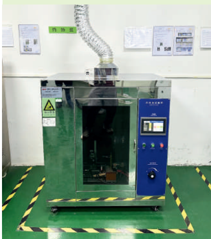
GLOW WIRE TESTER MACHINE
